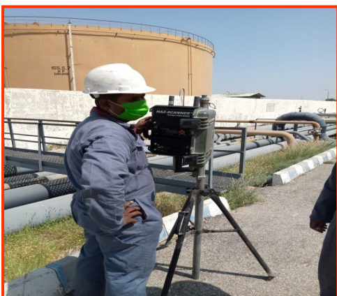
Fugitive Emission Testing
