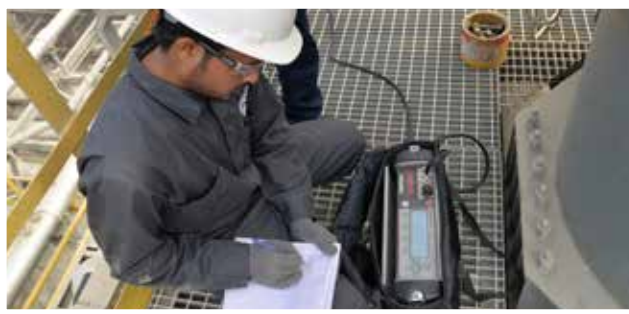
Stack Emission Testing
